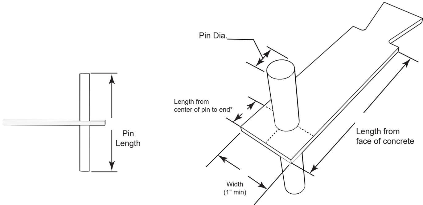
\*Pins are available loose or welded in place.
