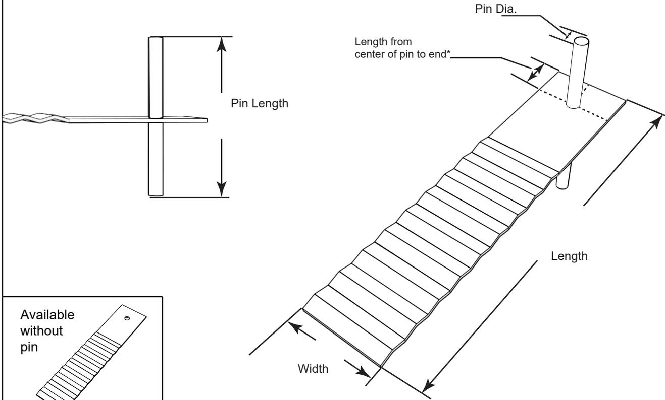
\*Pins are available loose or welded in place.
