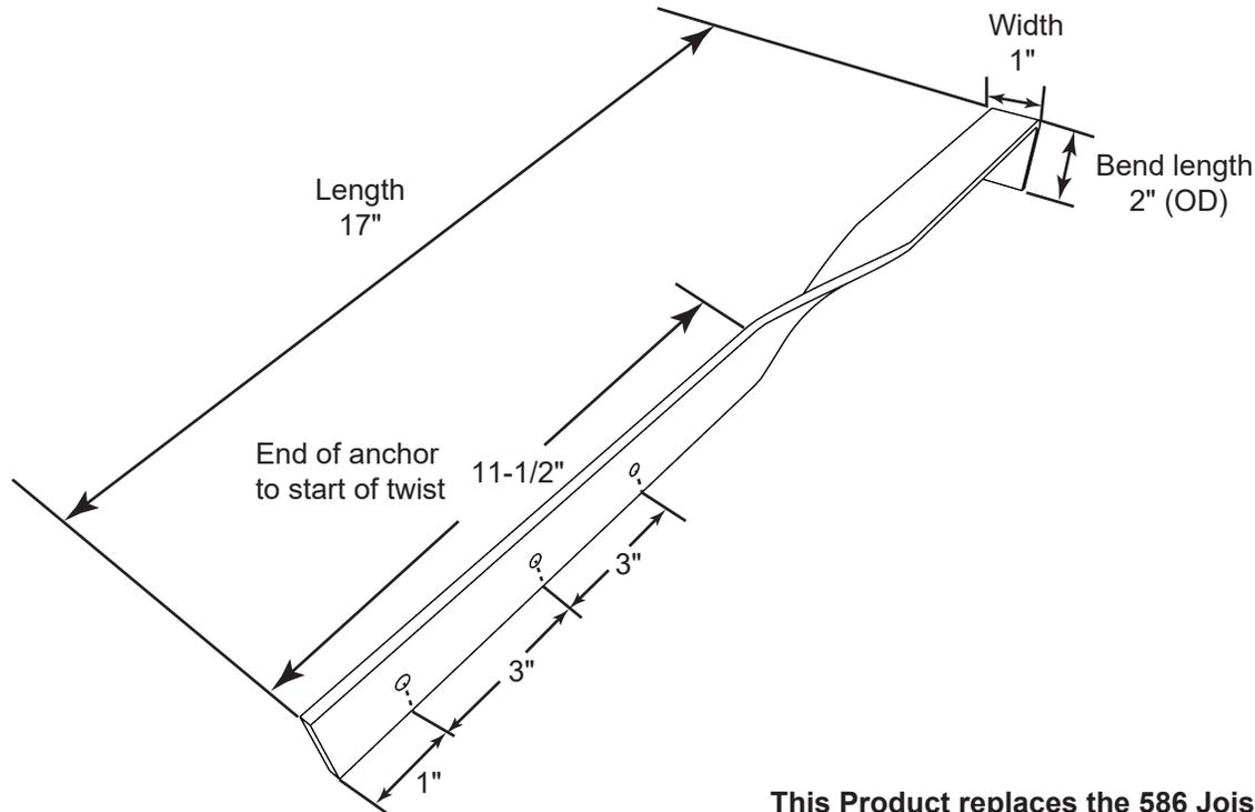
This Product replaces the 586 Joist Pin Anchor
